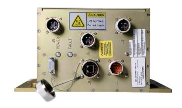
The network switch is a flange mounted device, utilizing an ARINC 763 enclosure. The external interfaces of the switch include three rectangular Quadrax connectors on one face of the enclosure for all PoE interfaces, and four circular connectors (one power/signal, three fiber optic) and a RJ-45 jack and RS232 connection on the opposite face.
